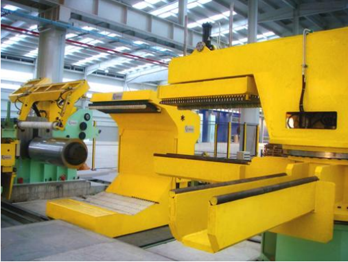
Surface type rolling Car on Recoiler for stainless strip 1500 x 3 mm & Strapping Capstan
