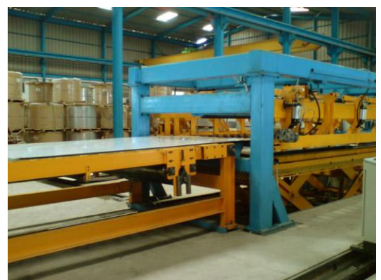
Inspection conveyor & Bomb-Door Stacker for 2000 x 12 mm stainless steel
