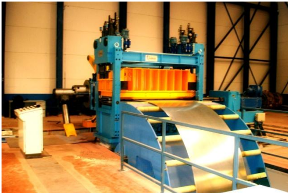
Precision Leveler machine of 3 + 3 highs for 2000 x 3 mm
