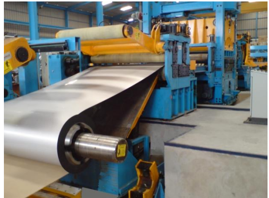
Decoiler & Inlet area of Cut to Length Line for Stainless Steel strip of 2000x12 mm
