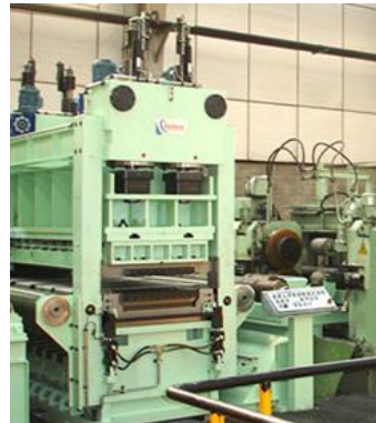
High Precision Leveler with top bridge balancing on 4 pivots for Stainless Steel 2000 mm. x 3 mm
