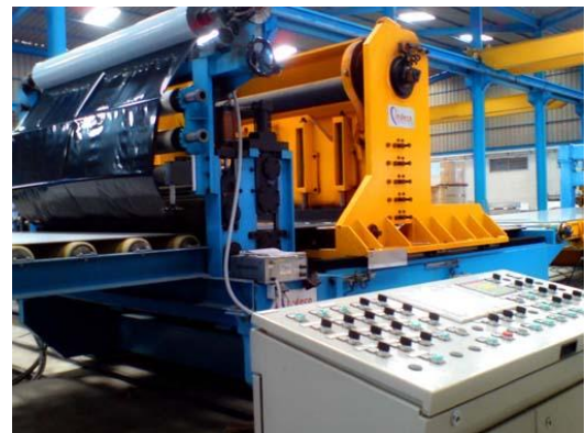
PVC film Applicator & Flying Shear for stainless strip 1500 x 10 mm
