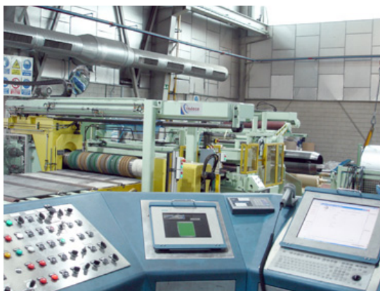
Control desk for Slitting line for stainless steel of 1500 mm. x 3 mm. x 150 m/min.
