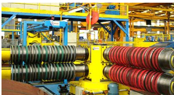
Slitter automatic tool change
