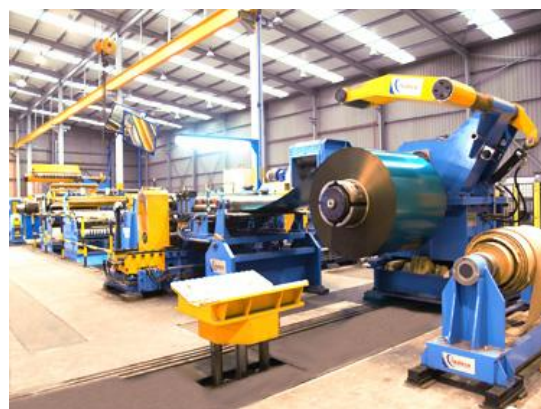
High performance Slitting Line of 1.250 mm. x 0,1 up to 3 mm of thickness x 350 m/min
