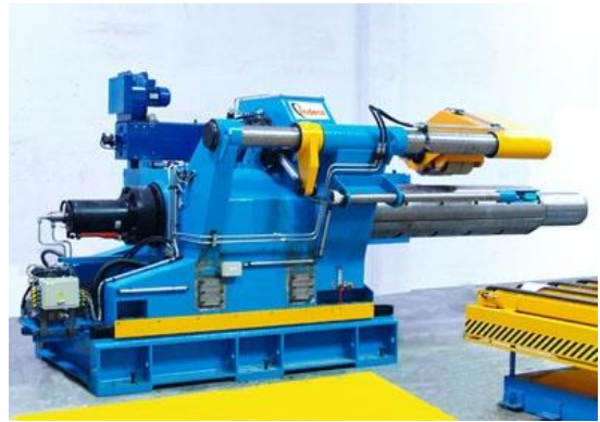
Hydraulic Decoiler for 40t. weight x 2000mm x 10mm. For Stainless Steel
