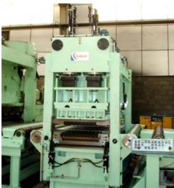
High Precision Leveler of 3+3 heights for stainless steel strip of 3 mm thickness x 2000 mm width
