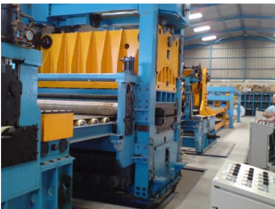
Precision Leveller for High Thickness for stainless strip of 2000x12 mm
