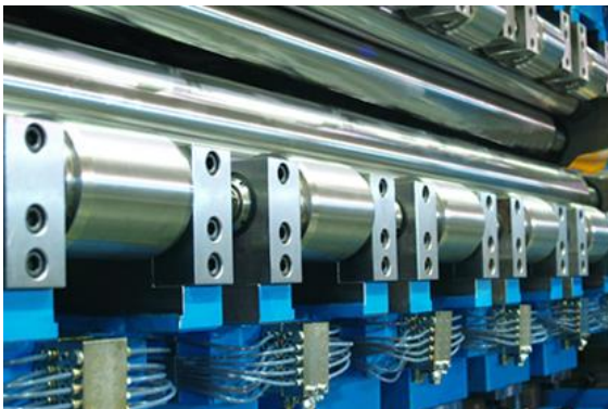
High Precision Leveler of 3+3 heights for stainless steel strip of 12 mm thickness x 2000 mm width
