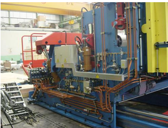
Erection of Hydraulic Piping on Desplaceable Tension Unit
