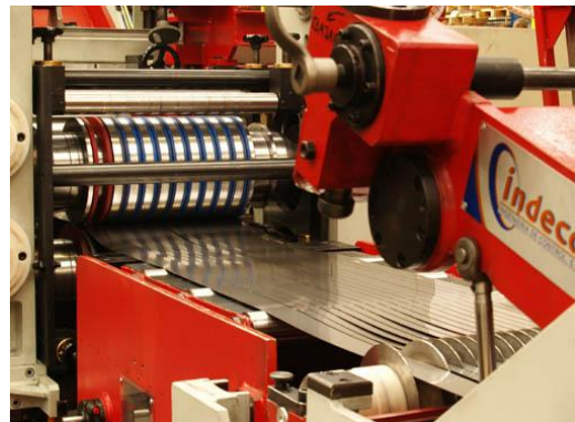
Detail of Slitter of 600 mm x 0,1 - 3 mm x 350 m/min
