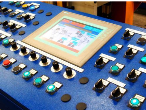
Last generation control system for slitter 600 mm x 0,1 - 3 mm x 350 m/min. - Stainless/Al/Cu/Brass
