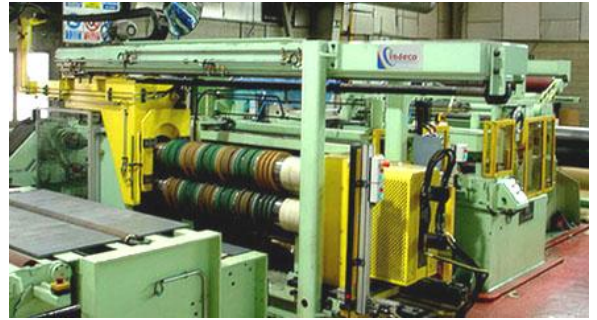
Slitting Line for stainless steel of 1500 mm x 3 mm x 150 m/min.
