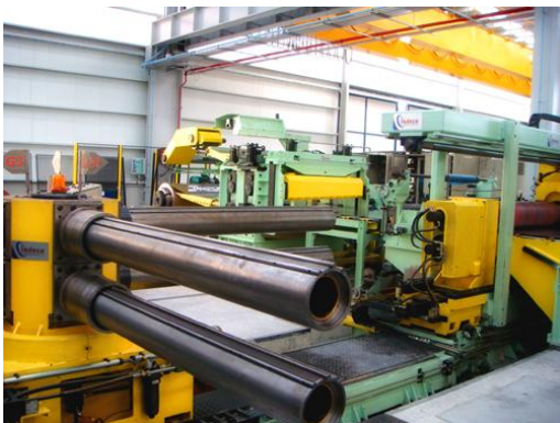
Slitter with automatic tooling change over (less than 5 minutes) for stainless strip 1500 x 3 mm
