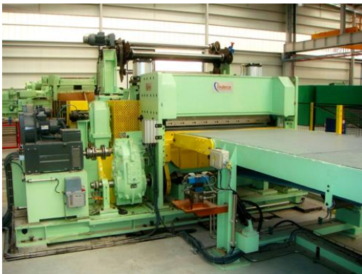
High Speed Electronic Shear (90m/min) 1500 x 3 mm
