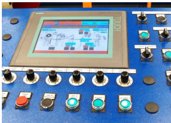
Last generation control system for slitter 600 mm. x 0,1 - 3 mm. x 350 m/min. - Stainless/Al/Cu/Brass.
