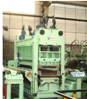
High precision leveler with top bridge balancing on 4 pivots. For Stainless St. 2000 mm x 3 mm
