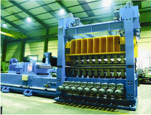
Counter rolls motor drive for precision leveler stainless steel 2000 mm x 8 mm
