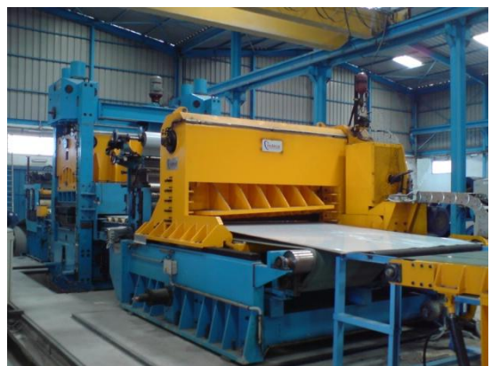
Flying Shear (50 m/min) for stainless steel strip 2000x 3 mm to 12 mm thicknesses
