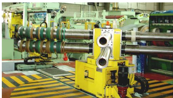
Slitter automatic tool change
