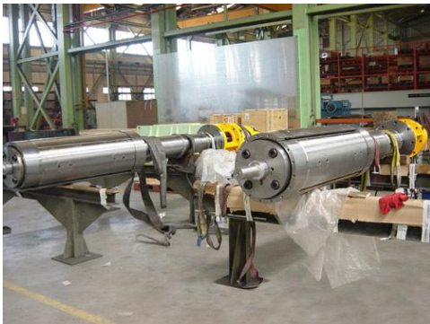
Erection of Rolls for Tension Leveler Unit
