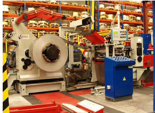
Decoiler & fully automatic strip centring system for 600 mm. x 0,1 - 3 mm. x 350 m/min
