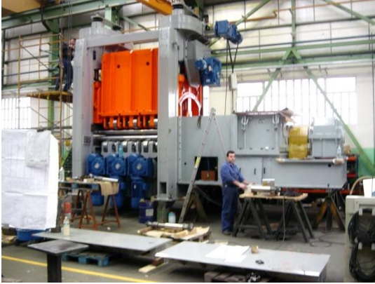
Erection of Precision Leveler for High thickness strip 2000 x 25 mm
