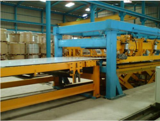
Inspection conveyor & Bomb-door Stacker for 2000 x12 mm for stainless steel 15 mm
