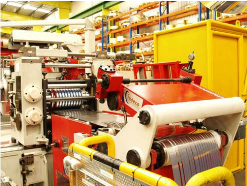
Slitter & Traction Rolls & Inlet basket for Stainless Steel 600 x 3 mm
