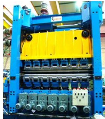
Counter rolls motor drive for precision leveler stainless steel 2000 mm x 10 mm
