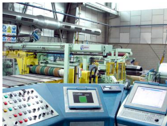
Slitting line for stainless steel of 1500 mm. x 3 mm x 150 m/min.
