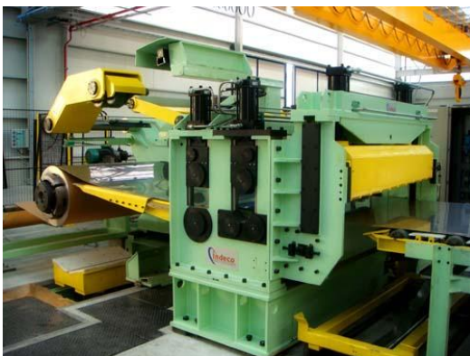
Straightening Rolls & Crops Shear for stainless strip 1500 x 3 mm
