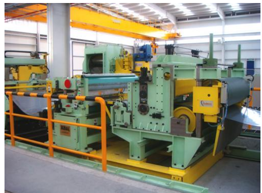
Rotary Belt Bridle & Displaceable Tension unit for stainless strip 1500 x 3 mm
