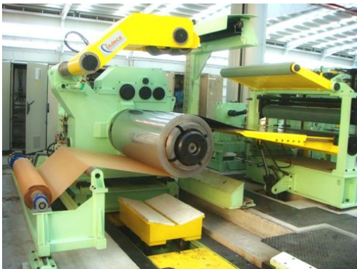
Decoiler & Inlet area of Slitter for stainless strip 1500 x 3 mm
