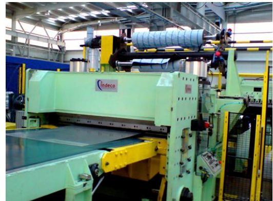
High speed Electronic Shear (90 m/min) for stainless strip for 1500 x 3 mm
