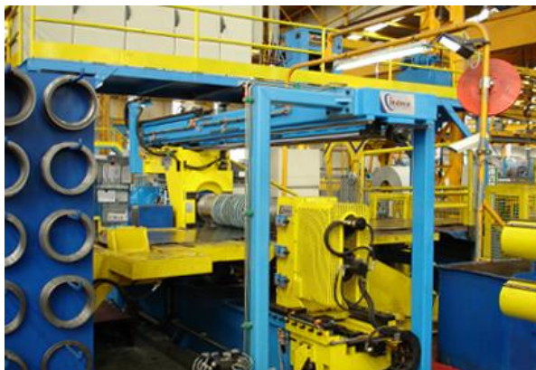
Slitting Line of 1500 mm x 6 mm x 200 m/min
