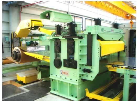
Decoiler & Straightener & Crops Shear for stainless strip 1500 x 3 mm
