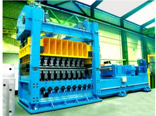
Counter rolls drive for High Precision Leveler for 2000 mm x 8 mm
