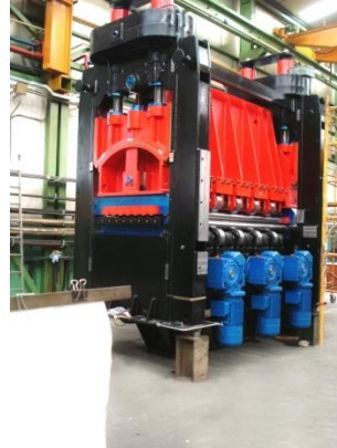
Erection of Precision Leveler for High Thickness for de 2000 x 25 mm
