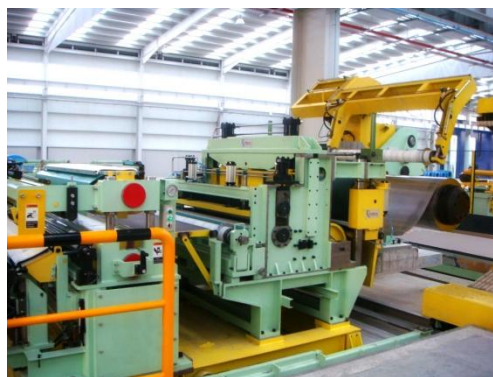
Rotary Belt Bridle & Displaceable Tension unit for Slitter for stainless strip 1500 x 3 mm
