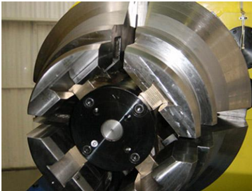
Detail of double decoiler for 40 t. and strip thickness of 15 mm
